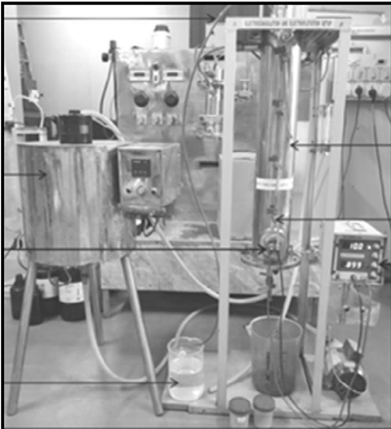
Fig. 1: Electrocoagulation and electrofloatation enhanced membrane module (ECEFMM)
